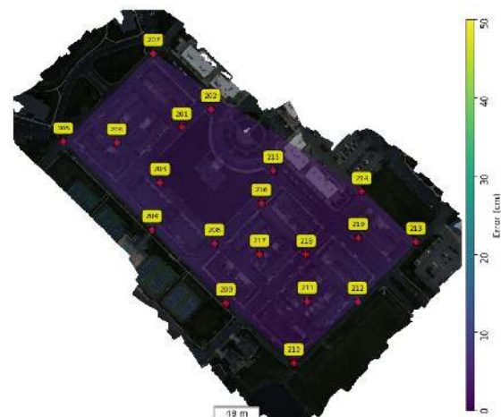
Visualization of the expected absolute position error within the checkpoint area.
